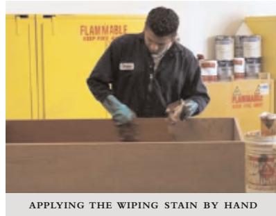
APPLYING THE WIPING STAIN BY HAND
