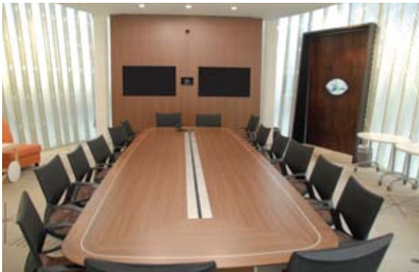
Technology wall and voice-power-data trough in table.
